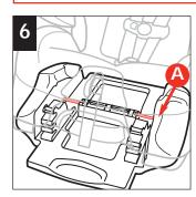
Reinstall Base: Remove bar from base. Line up shell with base. Begin with the rounded end, push bar completely through hole, starting on the right side (A), until it locks in place. Refer to "Removal of Seat Base".
